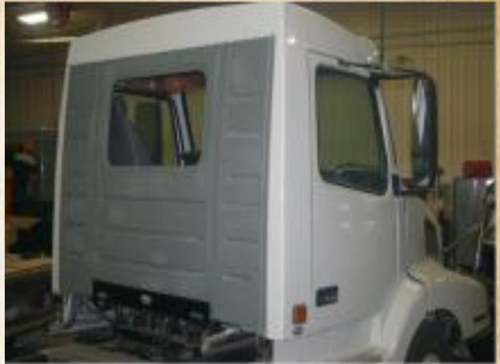
The standard Prairie Tech structural components have been adopted to provide for a rigid and sturdy cab. Reinforcement is included in the back panel to accept hardware for mounting cab extenders for those customers who wish to include that feature to enhance fuel economy. A new suspension is also included.
